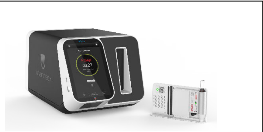
Figure 5. Prototype rendering of Myrna™. Myrna is a point-of-care instrument being developed to quantify InSep's 29 mRNA's using LAMP with a turnaround time of <30 minutes. PAXgene whole blood tubes can be inserted into a microfluidic cartridge without need for pipetting, and <2 minutes of hands on time is required.
